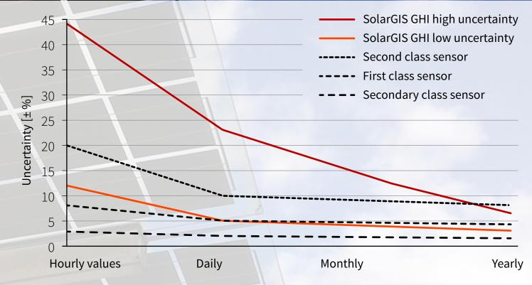
Comparison of satellite-based GHI data uncertainty with ground-based pyranometers (SolarGIS)
