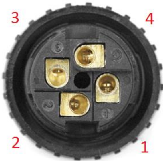
Figure 10a. Pin numbering in power connector
