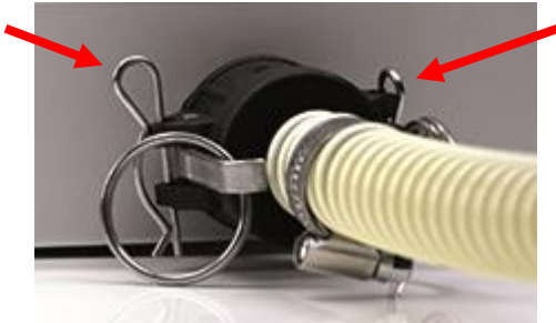
Figure 6: securing the Camlock
