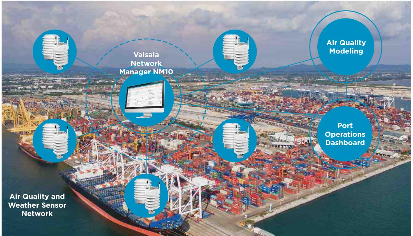
Vaisala Air Quality solution for ports consists of a network of compact air quality sensors and weather stations, complete with data acquisition and visualization software, as well as optional air quality dispersion modeling.
