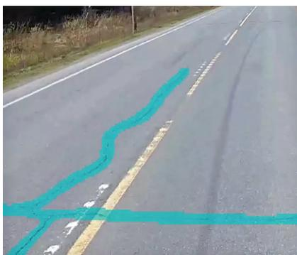
Automated visual inspection of road surface e.g. road markings, crackings and potholes.
