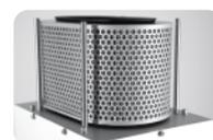
**PGS-100 Sun Photometer** is a radiometer that uses a solid state spectrometer with a CCD detector array to measure the direct solar radiation in the wavelength range from 350 nm to 1050 nm. The only maintenance is to periodically clean the optical window and check the desiccant in the radiometer. The PGS-100 must be mounted on an automatic sun tracker to make measurements. Mounting kits are available for the Kipp & Zonen SOLYS 2 and 2AP sun trackers.
