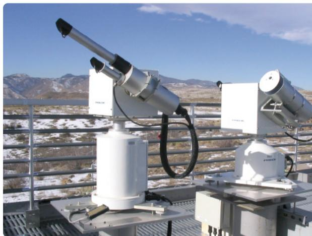
POM-O1 and POM-O2 are installed around the world for reliable automatic solar radiation measurements in meteorology, climatology, atmospheric chemistry and pollution studies. POM is the basis of the Asia-Pacific SKYNET network for aerosol monitoring and satellite ground-truthing. Parameters such as optical depth, scattering coefficients, aerosol distribution and energy distribution can be derived from the data.
