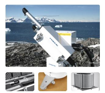
**PGS-100 Sun Photometer** is a radiometer that uses a solid state spectrometer with a CCD detector array to measure the direct solar radiation in the wavelength range from 350 nm to 1050 nm. The only maintenance is to periodically clean the optical window and check the desiccant in the radiometer. The PGS-100 must be mounted on an automatic sun tracker to make measurements. Mounting kits are available for the Kipp & Zonen SOLYS 2 and 2AP sun trackers.
