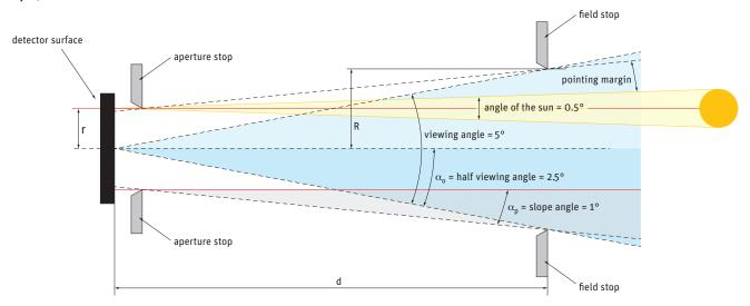
For the SHP1 the full viewing angle is 5 °, the slope angle is 1 °. The sun, as seen from the detector, occupies a solid angle of 0.5 °. A 100 % response can be expected only if the sun is entirely within the slope angle. This is the case when tracking accuracy is better than slope angle minus half the solar angle.
