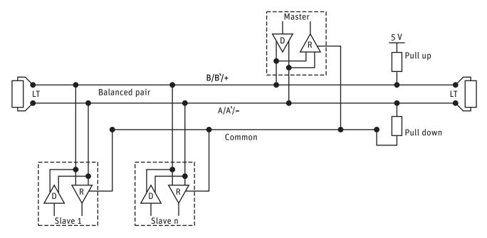
The interface needs also an external power to provide the voltage for the electronics. If the interface is the last device on the network then a terminator consisting of a  $120\Omega$  or  $150\Omega$  resistor has to be connected between terminal A/A'- and B/B'+. Never place the line termination on the derivation cable. It is required to install the pull up and pull down resistors as shown in the previous figure. The value of these resistors has to be within  $650\Omega$  and  $850\Omega$ .
