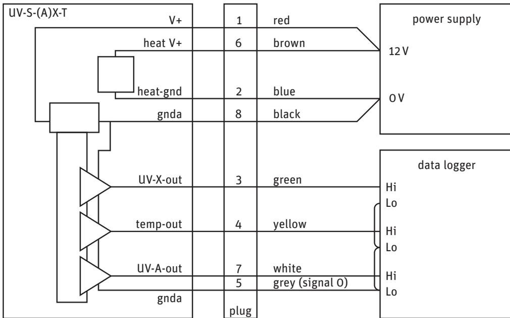
**Note** Pin 3 [green wire] is the UV-B or UV-E output
