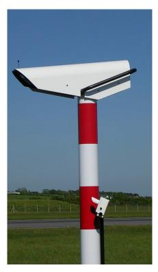
LM21 measures the ambient light level or background luminance in RVR applications. In the picture, LM21 is installed on Vaisala Transmissometer LT31.
