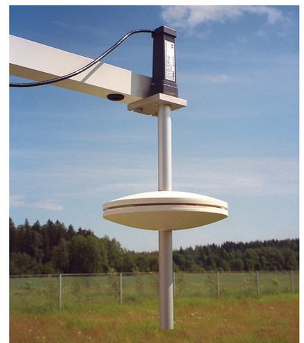
PTB210 paired with SPH10 static pressure head
