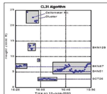
Figure 1. Basic operation of Sky Condition Algorithm. The new algorithm computes in 2D time-height domain.
