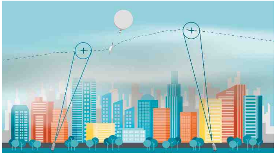
Ceilometers provide a vertical dimension to air quality monitoring by reporting the MLH. Typically, a low MLH indicates that the pollution level is high as the pollution is concentrated into a smaller volume.
