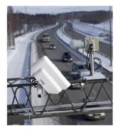
state sensor provides a value of grip that gives decision makers a quantitative reading of the current road slipperiness. This grip value can be used for a variety of decision-making tools, such as performance indexes or a trigger for variable message signs.
