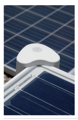
**rt1** is a small, fully weatherproof duo-sensor that independently measures the incoming solar irradiance and the back panel temperature. Thanks to this included back panel temperature sensor you collect all the data you need to monitor the performance of your installation - all in digital Modbus® format. Thanks to the unique design you can easily fix it to your PV panel without the need for any tools.
