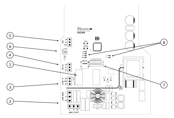
Figure 2: Main circuit board of the light head
