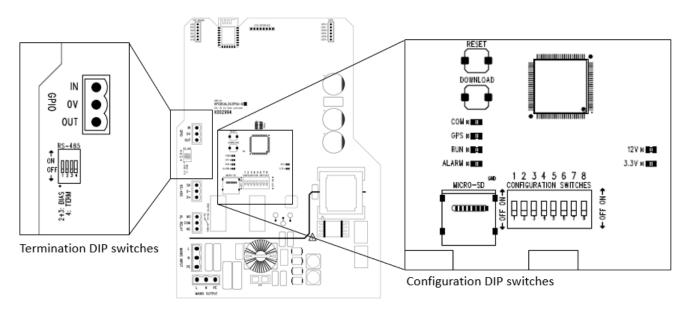
Figure 8: Location of the DIP switches
