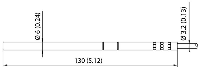
PTU30T for pressure and temperature only measurement
