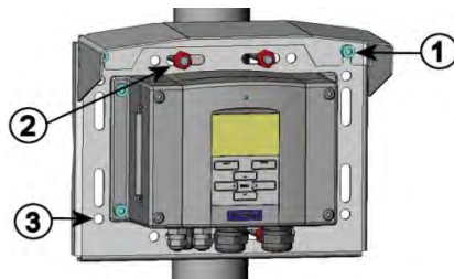
Figure 15 Mounting Rain Shield with Installation Kit
