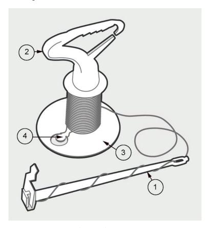
Figure 5 RS41 Unwinder Details
