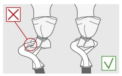
3. Align the unwinder so that it points directly downwards from the balloon neck, as illustrated in the figure below.
