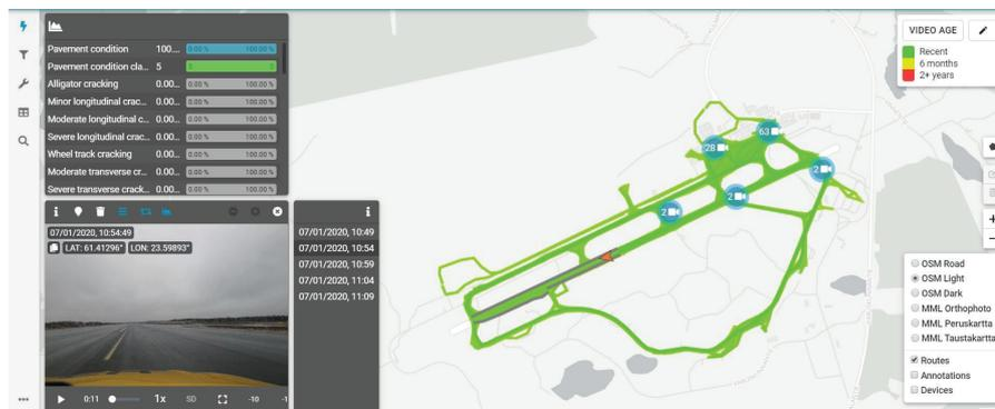
**RoadAI makes it easy to collect, view, and leverage runway condition data on a map.**
