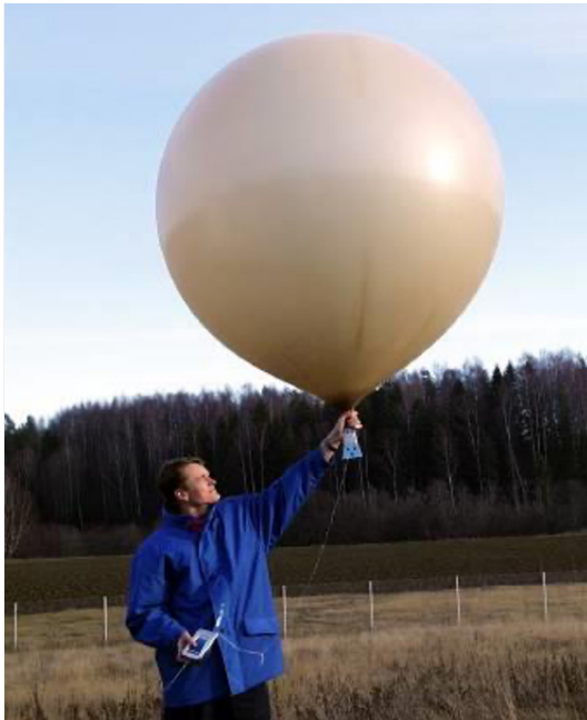
Attached to the balloon is a radiosonde, which relays data from the upper atmosphere to the ground. This data is one of the key measurements of weather forecasting.
